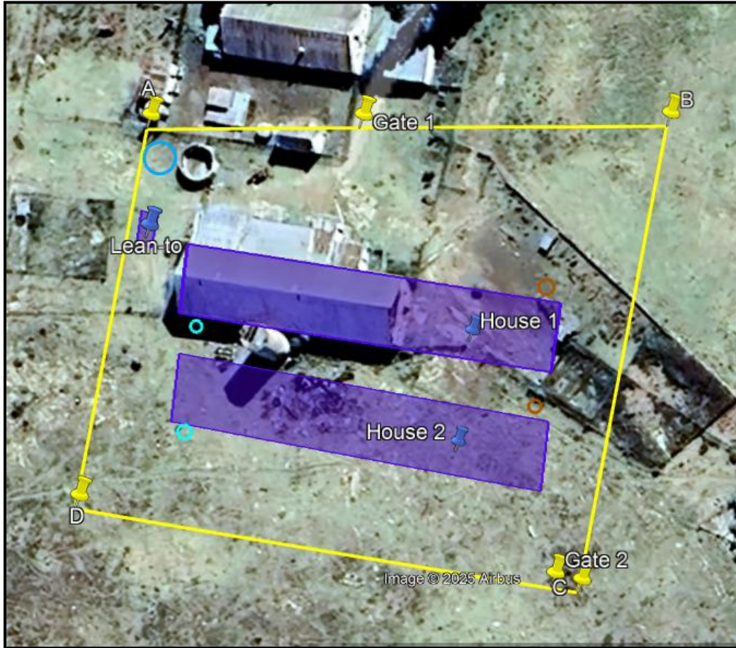
Figure 2: Schematic representation of the development after expansion where the blue polygons indicate the layer houses and lean-to, the blue circles show the JoJo tanks and cement dams, and the brown circles indicate the feed silos. The yellow line indicates the fenceline of the facility.
